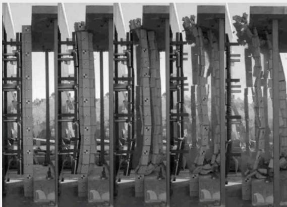
Unreinforced masonry wall under blast load
